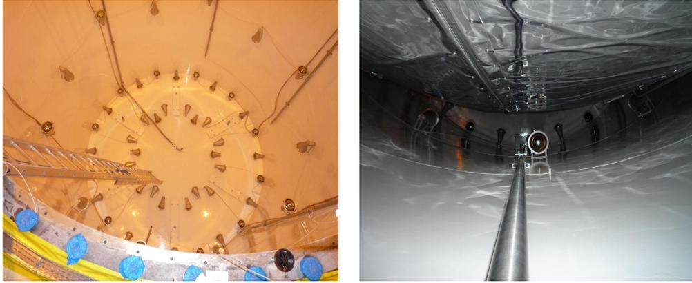
Figure 3.18: Photograph of the Inner Veto vessel, on the left, from its PMT installation period. On the right it is a picture taken after the ID installation, where the Buffer vessel and its reflective wall can be seen.
