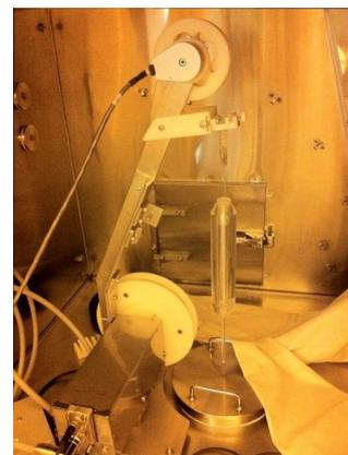
Figure 3.25: Picture of the Double Chooz Far Detector Glove Box, on the left, and  $z$ -axis deployment system, on the right.
