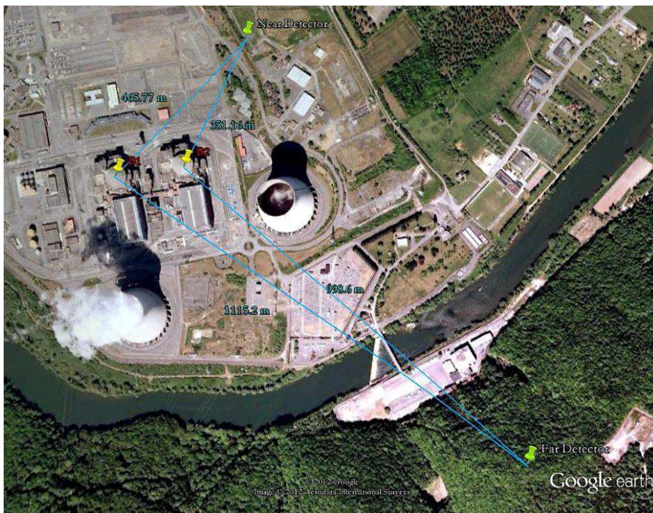
Figure 3.2: Satellite photograph of the Double Chooz site in Ardennes, France. The two Chooz B reactors are marked with yellow pins while the Near and Far detectors are indicated with green pins. The blue lines are the baseline of each detector to each reactor.
