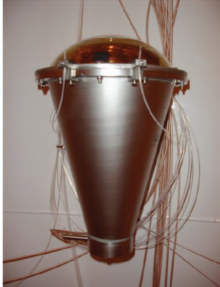
Figure 3.28: Two fibers attached to an IV PMT.
