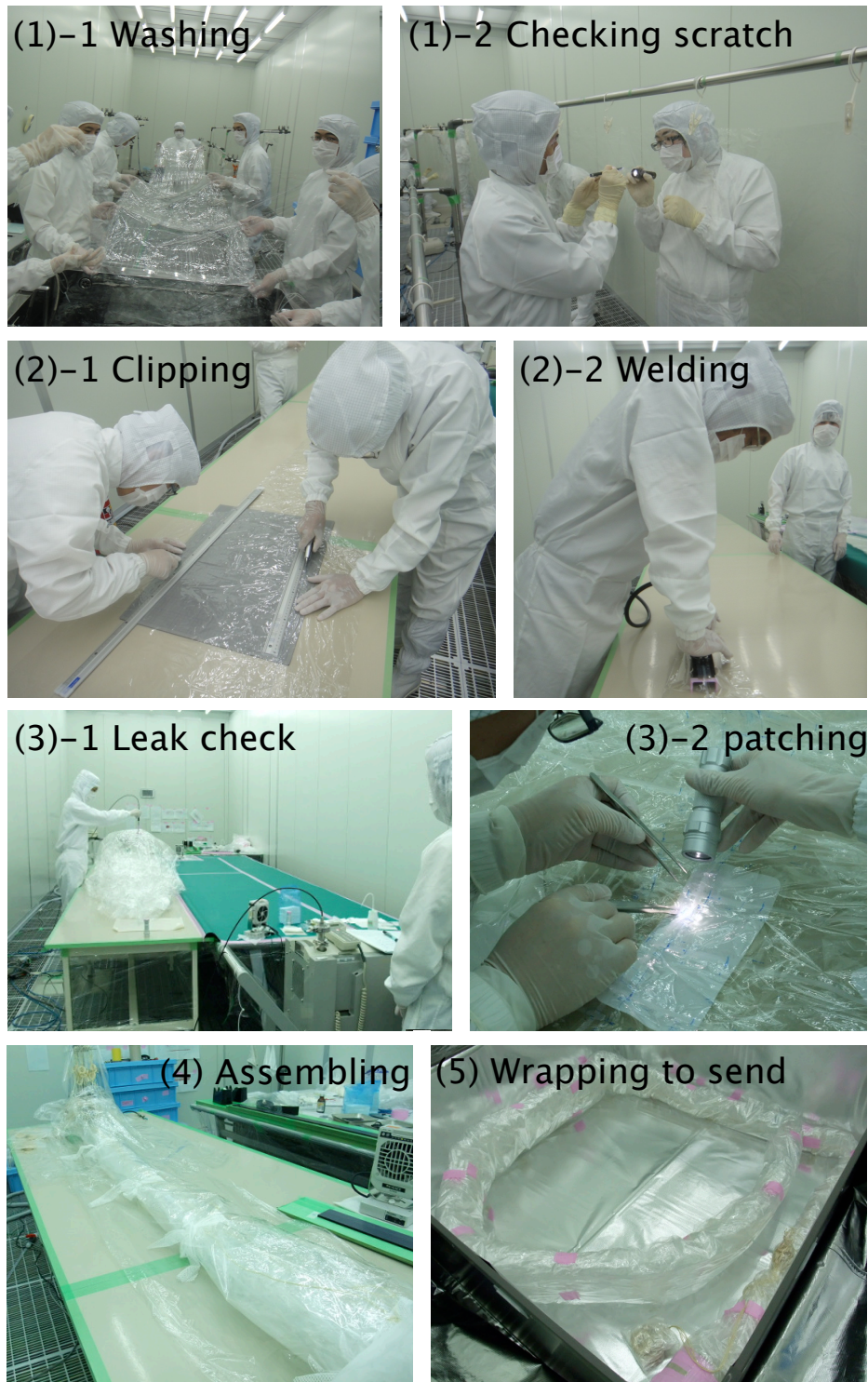
Figure 3.15: Pictures of the IB fabrication. [(1)-1] The film washing by the ultrasonic cleaning with pure water. [(1)-2] Checking scratches/pin holes by eyes. [(2)-1] Clipping the gores. [(2)-2] Welding. [(3)-1] Leak check with helium detector. [(3)-2] Patching the film with glue. (4) Assembling the IB, connection pipe, supporting belts and Vectran strings. The IB covered with inner envelopes. (5) The wrapped IB in the plastic box. The box covered with an air tight bag and filled N_2 . It sent to the experimental site.
