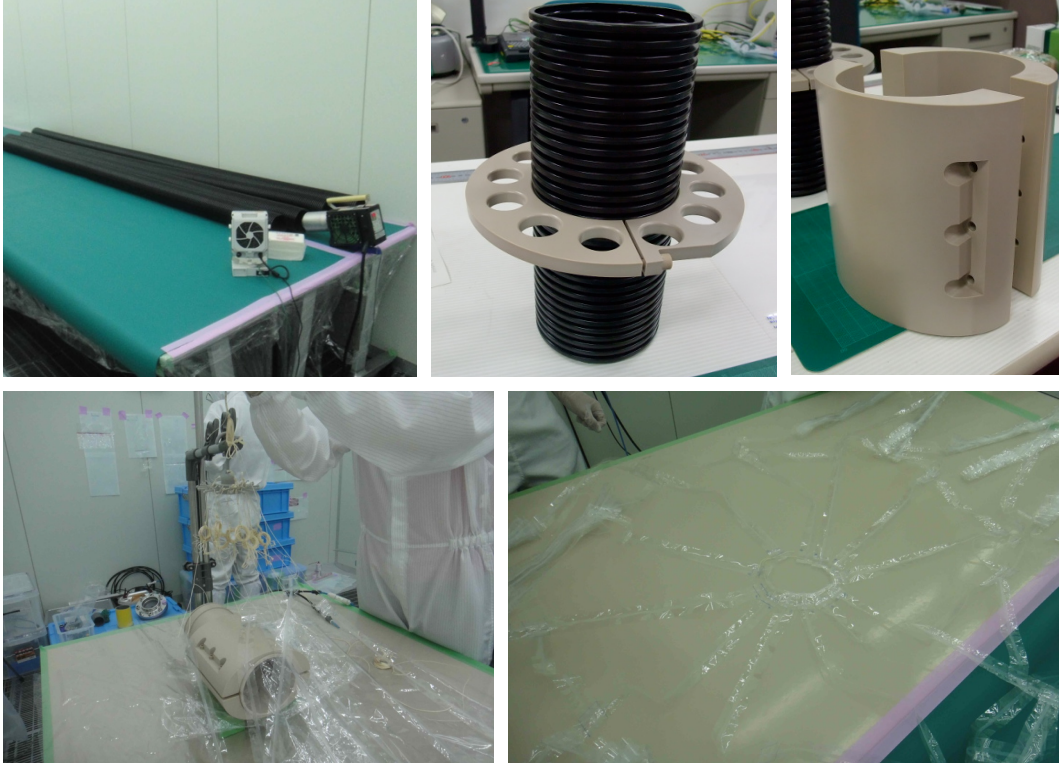
Figure 3.14: Pictures of supporting structures. Corrugated nylon tube cut in a \sim 2 -m-pieces and made it straight by a heat blower (top-left). String guide (top-center). Connection pipe made of PEEK material (top-right). Film belt with Vectran strings (bottom left). Film belt structure at the polar (bottom-right).
