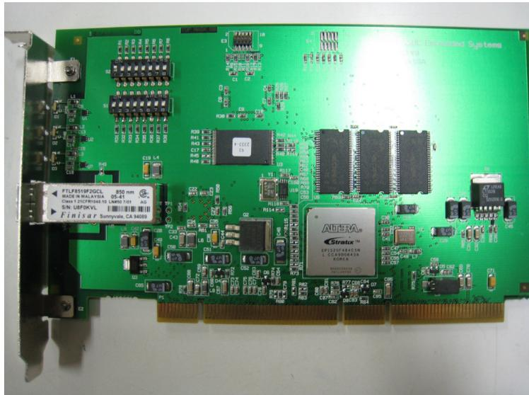
図 5.4 Reflective Memory: PCI-5565PIORC-110000 by GE FANUC
