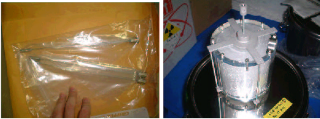
Figure 6.8: The devices of calibration source box. The left picture is devices of Ge, Zn and the right is for Am/Be.
