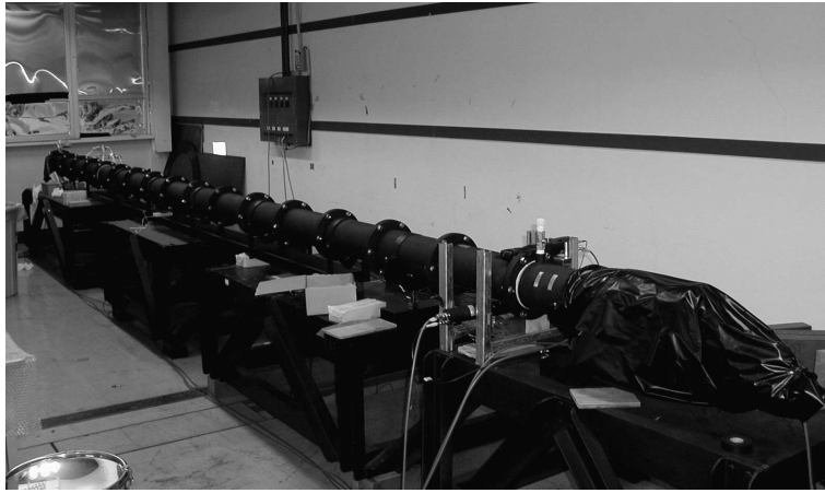
Figure 5.1: The picture of the setup apparatus for the light yield measurement.
