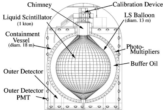
FIG. 1. Schematic diagram of the KamLAND detector.
