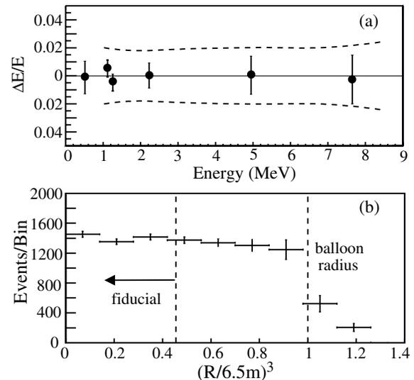
FIG. 2. (a) The fractional difference of the reconstructed average energies and known source  $\gamma$  energies. The dashed lines show the adopted systematic error. (b) The  $R^3$  vertex distribution of 2.2 MeV neutron capture  $\gamma$ 's. The level of uniformity over the fiducial volume is used in the estimate of the fiducial volume uncertainty.
