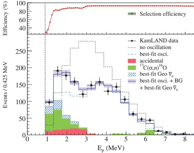
FIG. 1 (color). Prompt event energy spectrum of  $\bar{\nu}_e$  candidate events. All histograms corresponding to reactor spectra and expected backgrounds incorporate the energy-dependent selection efficiency (top panel). The shaded background and geo-neutrino histograms are cumulative. Statistical uncertainties are shown for the data; the band on the blue histogram indicates the event rate systematic uncertainty.
