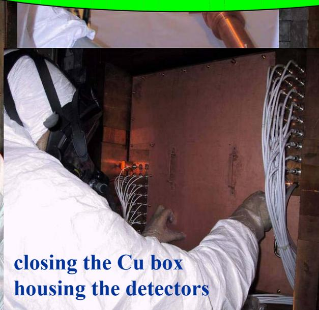
closing the Cu box housing the detectors
