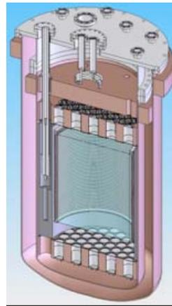
**SIGN:** A High-Pressure, Room-Temperature, Gaseous-Neon-Based Underground Physics Detector (100 kg @ 100 atm towards 10 tons)
