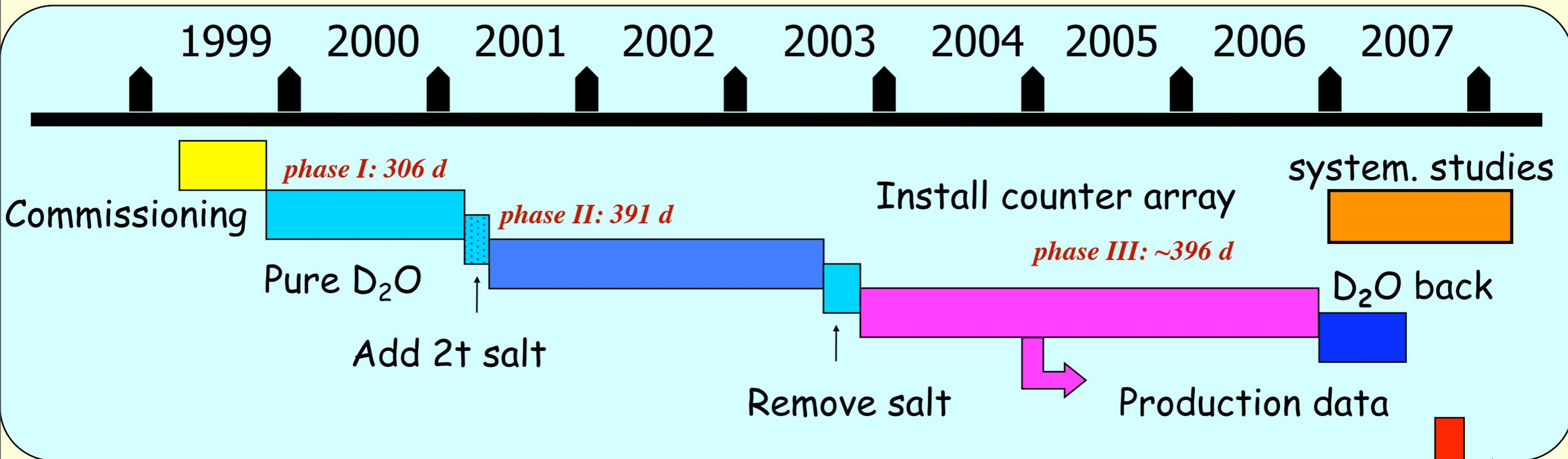
3 phases with different ways to detect neutrons
