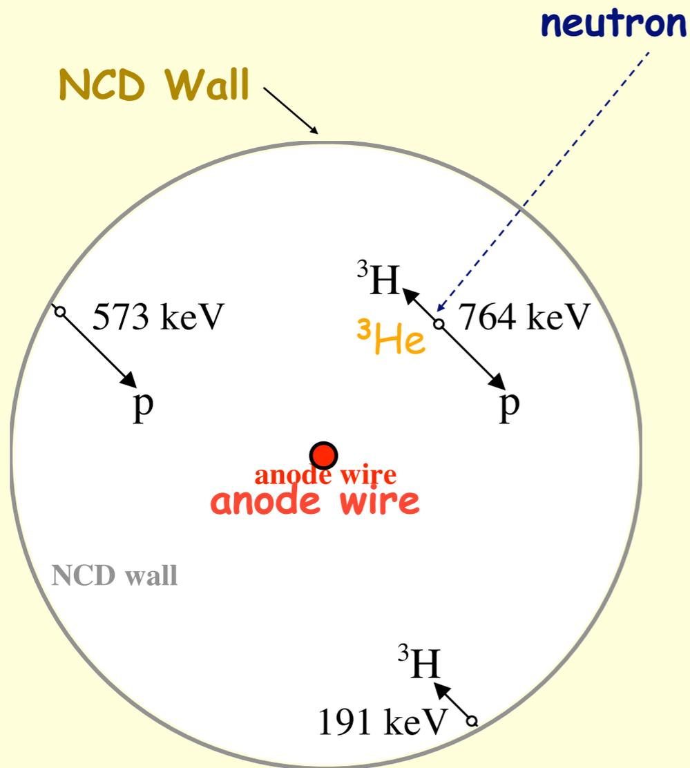
End view of an NCD with representative ionization tracks
