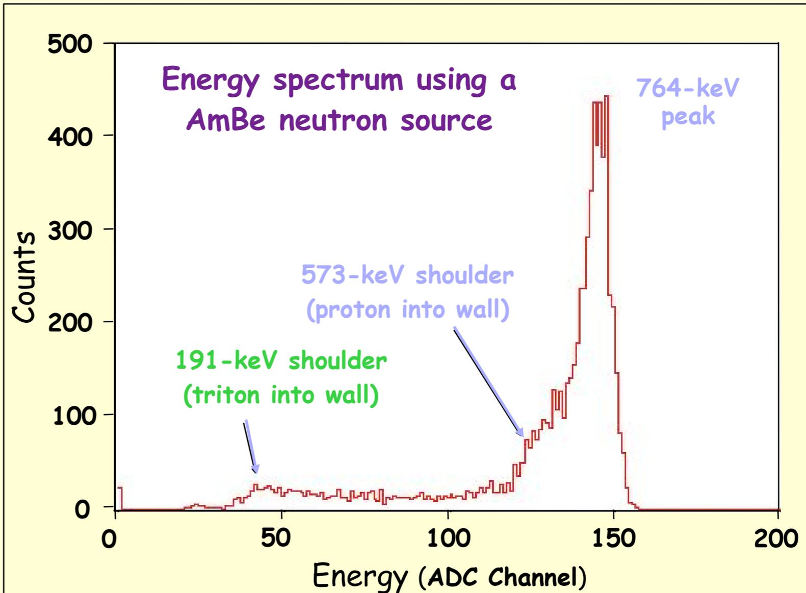
Energy spectrum from a single deployed  ${}^3\text{He}$  proportional counter. The main peak corresponds to the 764-keV Q-value of the  ${}^3\text{He}(n, p){}^3\text{H}$  reaction.
