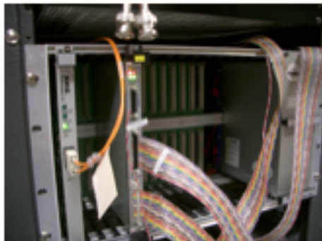
Figure 2: Backup trigger VME crate
