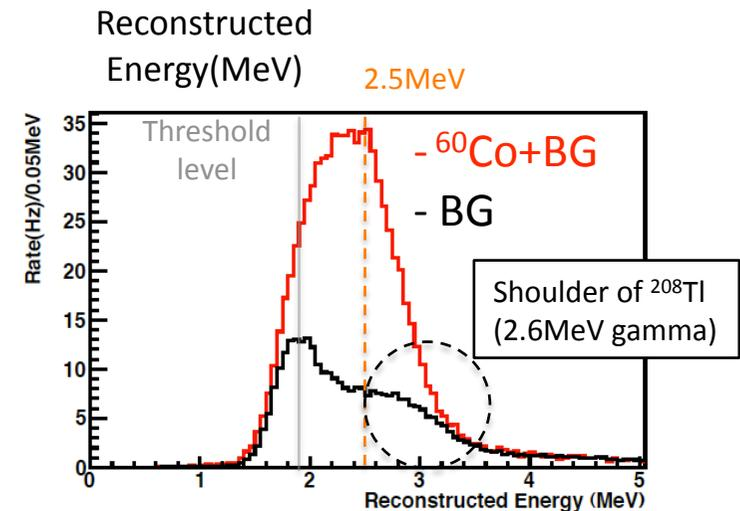
Now the energy scale has been calibrated roughly with 2.5MeV peak of the total charge distribution for the  $^{60}\text{Co}$  source data.
