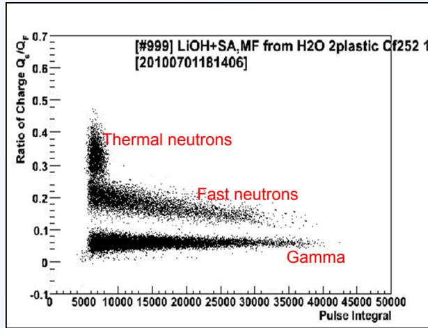
Triple PSD obtained in a Li-containing liquid mixture
