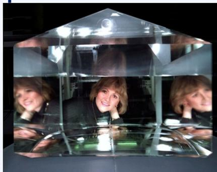
Technique used for rapid growth of NIF KDP crystals
