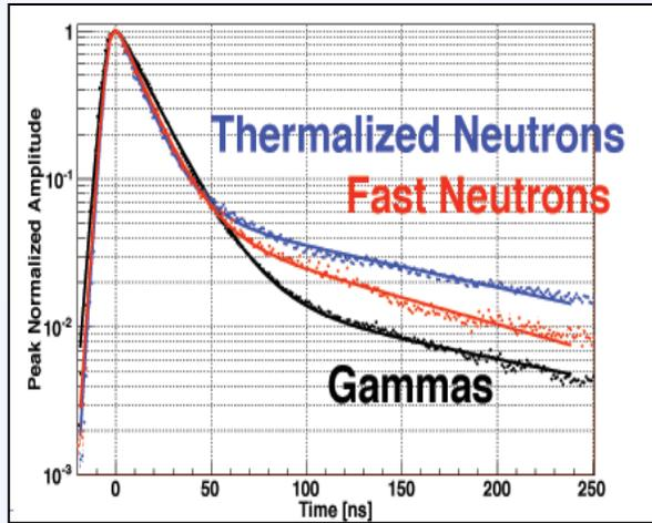
Triple PSD measured in a Li-containing single crystal
