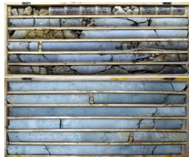
FIG. 2: Borehole rock samples from the near and far detector sites. (top)the sample in the near site entrance, (bottom)the sample in the far site.
