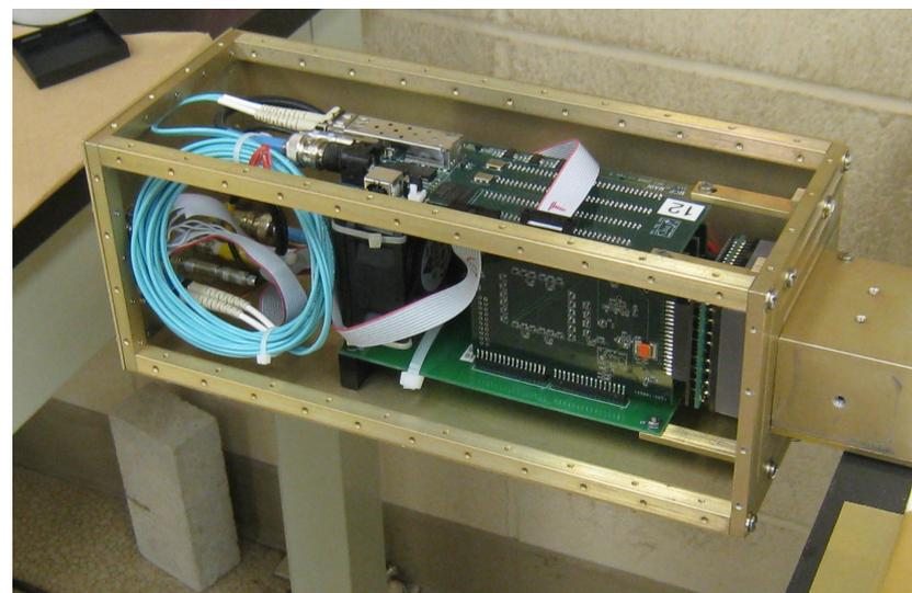
Fast waveform digitizer for the Photonis MCP is currently under development evolving from existing technology used in BELLE, BESS, ANITA. Length beyond photo-sensor will be ~125mm. One module per MCP.
