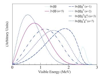
FIG. 1. (Color) KamLAND-Zen visible energy spectra for different <sup>136</sup>Xe decay modes, characterized by the spectral index *n*. The resolution-limited line [ $\sigma = (6.6 \pm 0.3)\%/\sqrt{E(\text{MeV})}$ ] at the *Q* value indicates the  $0\nu\beta\beta$  decay peak without Majoron emission.
