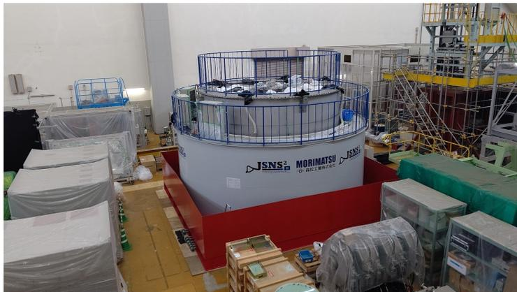
Figure 3.2: An entire viewing photo of the detector at HENDEL building. The red-painted square shape wall is anti-oil-leak wall welded on the edge of the tank base. The outer cylindrical structure with JSNS<sup>2</sup> logo on the surface is the 1-st anti-oil-leak wall. The most inner and highest structure is the s.s.tank of the detector. There are ladders and decks on the 1st anti-oil-leak tank for accessing to the detector.
