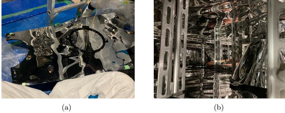
Figure 3.12: (a) A photo of the reflection sheet attached to the black board. (b) A photo of the top lid veto layer after installation. One can find that most of the surfaces, such as the PMTs, the s.s.tank, and the optical separator, is covered with reflections sheet.
