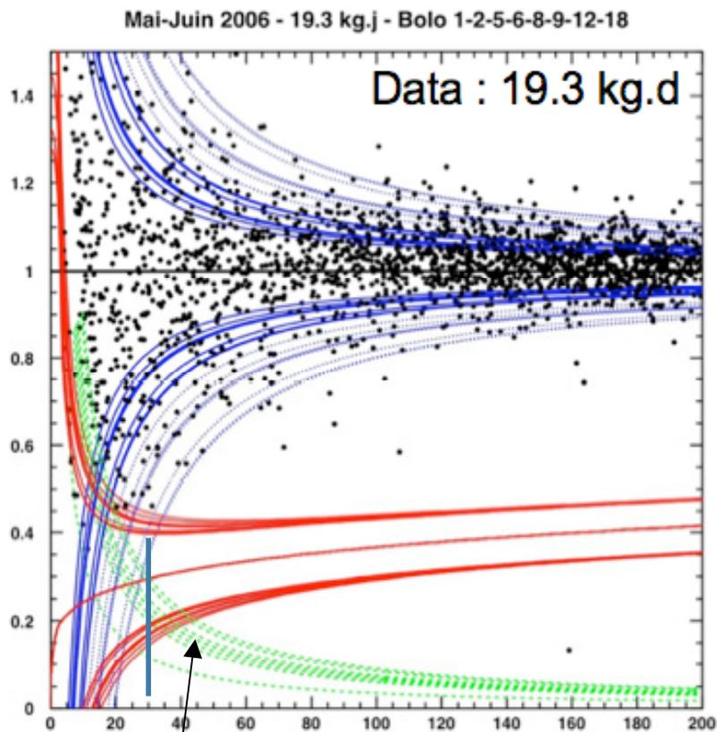
Er thresholds of 8 detectors (from 20 to 35 keV)
