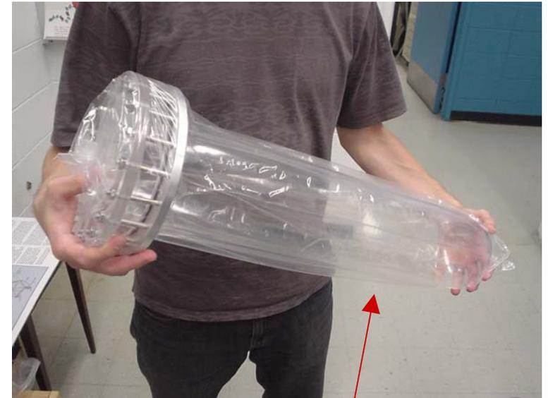
20 kg synthetic fused silica vessel, sealed against exposure to Rn
