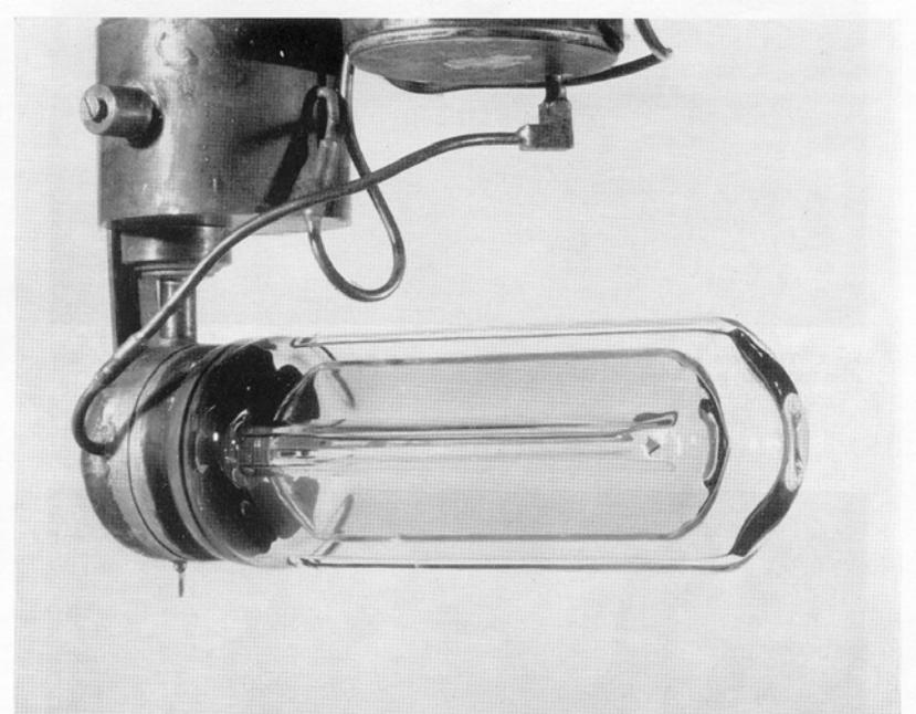
Fig. 2. Assembled bubble chamber and jacket.
